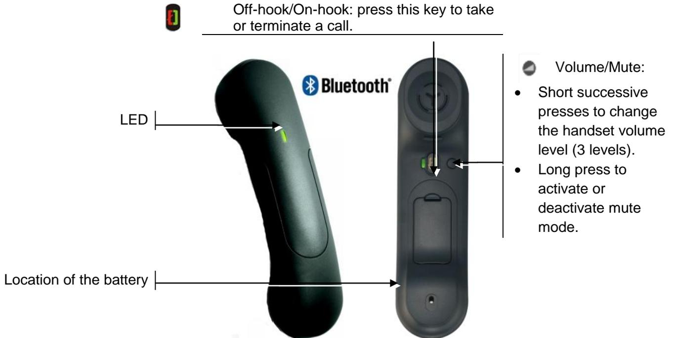
If the Bluetooth® handset is on its base, you do not need to press the Off-hook/On-hook key to take or terminate the call. Just off-hook/on-hook the Bluetooth® handset.
