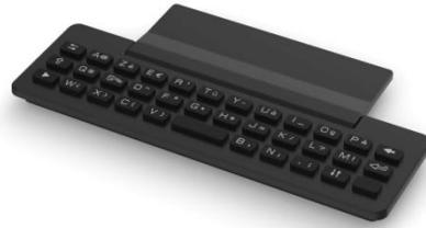
Use the keyboard to enter names while configuring the phone. Directly access the dial by name feature by entering the name of your caller on the keyboard.
