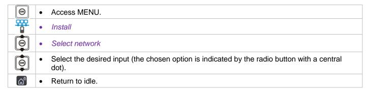
The selection is retained even after switching the telephone on/off. The selection of a specific system (SYSTEM...) forces operation on a specific system. This selection must be changed if one wishes to change system. Selecting 'Auto. select' enables the telephone to connect automatically when it enters a system coverage zone. If the systems programmed in the telephone have common coverage zones, the telephone selects the first system found.
