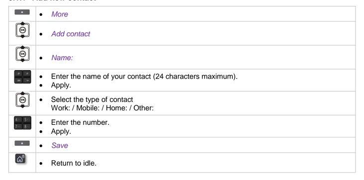
To key in the name: the keys in the numeric keypad include letters that you can display by pressing them successively. Example: press twice in succession on 8 to display the letter 'U'. To insert a pause in a number, press the 1 (hold down for a few seconds). To insert a measured break, press 0 (hold down for a few seconds). Press the # key to switch from lowercase letters mode to uppercase letters mode, and from uppercase letters mode to numbering mode.
