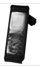
Your telephone can also be carried in a protective case with swivel clip (not supplied with the phone, please contact your installation technician). It is recommended to use the protective case if your telephone is to be used in an industrial environment (presence of dust, filings, vapors of diverse origins or its at the risk of being dropped). To avoid losing your telephone, get into the habit of clipping it onto your belt.
